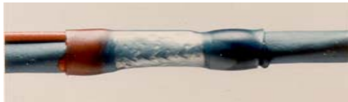
Acceptable: Fillet is clearly visible between the lead and shield.
