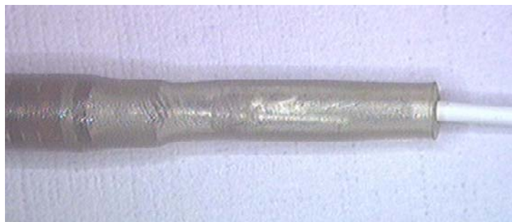
Acceptable: Solder has lost all appearance of ring shape. There is a definite fillet visible along the wire interface.
