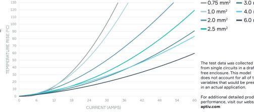
from single circuits in a draft free enclosure. This model does not account for all of the variables that would be present in an actual application.
