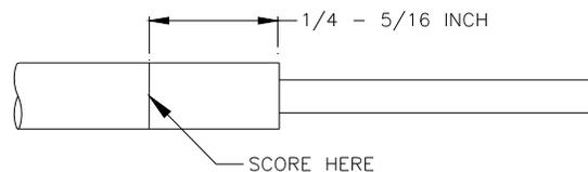
5. Remove section of jacket carefully by pulling straight. This will flatten the braid strand ends.
